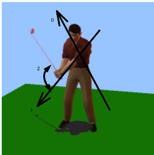
Figure 5: Mathematical model for the swing motion analysis (3 degrees of freedom)
